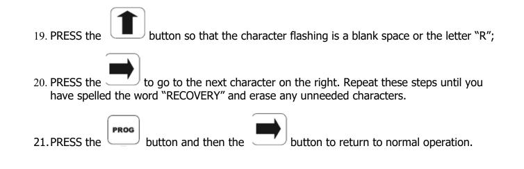
When selecting "RECOVERY" if above 285 degF "TOO HOT" will be displayed. When the temperature is correct "RECOVERY" will remain displayed. You are now ready to follow the RECOVERY PROCEDURE.
