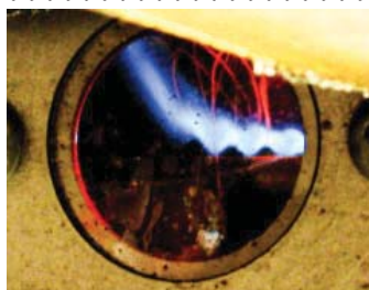
Lifting flame with too much air
