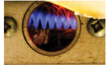
Lifting flame with lack of air
